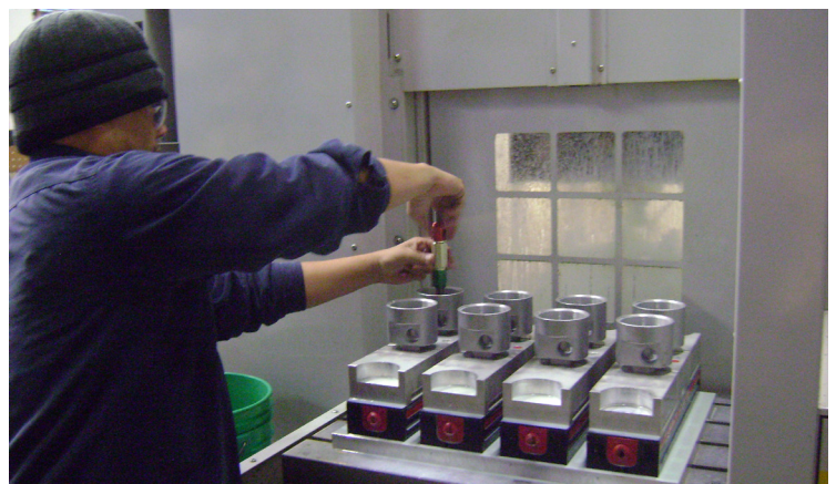
Parts for a hydroelectric plant are first turned on the SL6 slant bed turning center and then finished on the TT24 twin table machining center.
