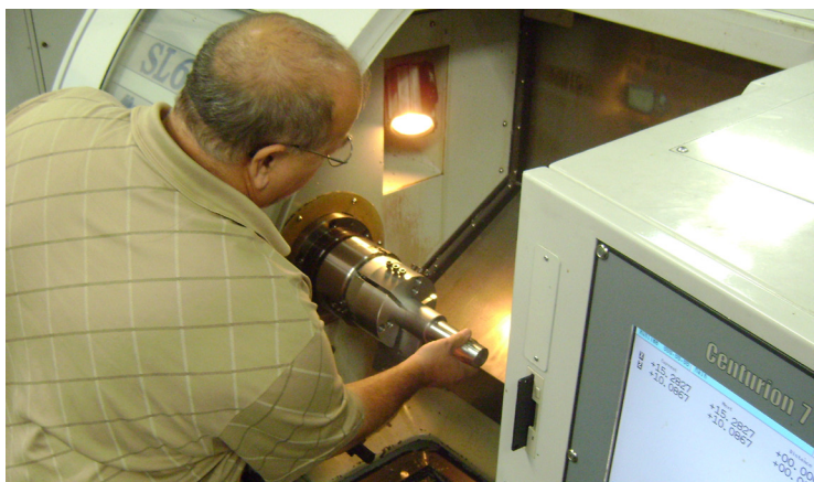
Parts for a hydroelectric plant are first turned on the SL6 slant bed turning center and then finished on the TT24 twin table machining center.
